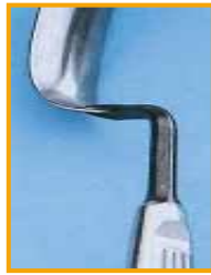
Retractors with discolored black shaft in hardened Cr-steel with the handle and blade remaining bright, made from non-hardenable CrNi steel.
