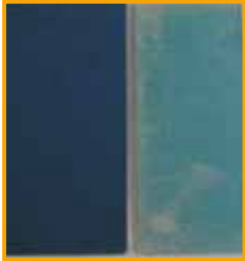
Left: Original Right: Optical changes to color anodized aluminum
