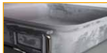
Severe material attack on the natural and color anodized aluminum surfaces of an instrument stand and containers. Cause: Overdosing of the otherwise material-compatible alkaline wash solution.
