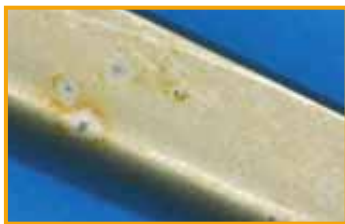
Pitting induced by chlorides on instrument
