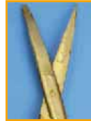
Corroded scissors made of stainless steel. Cause: Subsequent damage due to an acid attack caused by overdosing of the basic detergent.
