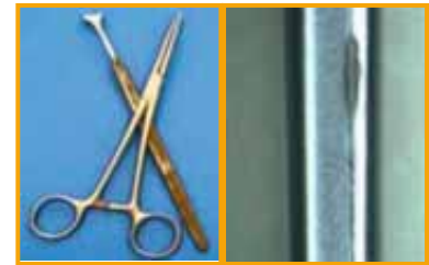
Contact corrosion: Stainless steel/Brass
