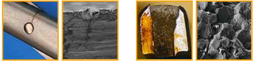
Detail: Scissors hinge joint with typical intercrystalline crack.
