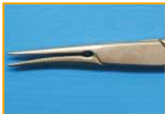
Deformation caused by improper handling
