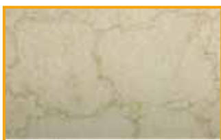
Marbling caused by impurities in steam condensate
