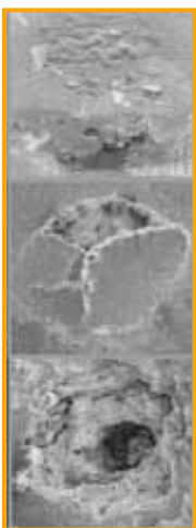
Scanning electron microscope image, chloride-induced pitting
