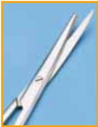
Scissors with broken tip. Cause: Incorrect loading
