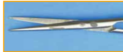
Left: Partial material attack due to acidic cement remover, and on the right due to a hemostatic agent. Cause: Excessive contact period or insufficient removal after use.
