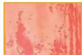
Severe material attack on the natural and color anodized aluminum surfaces of an instrument stand and containers. Cause: Overdosing of the otherwise material-compatible alkaline wash solution.
